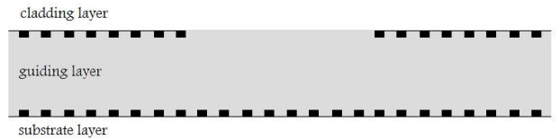
Fig. 4. Optical cavity with plasmonic diffraction grating
