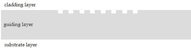
Fig. 1. Waveguide structure with diffraction grating
